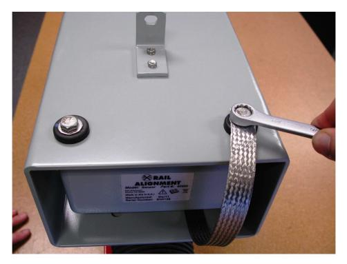
Next, install the sensor into the mount. Use the 5/16-18 x 1 1/4" Bolt provided with the kit to hold the strap in right rear position of the sensor as pictured above. Install the 5/16" internal tool lock washer onto the bolt, then the strap, then the flat washer that was originally provided. Tighten all four mounting bolts using a 1/2" wrench.
