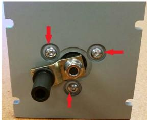
The pictures above show you the isolators (red arrows) that MUST be in place and in good physical shape when a new motor is installed. Without these isolators you will blow the motor fuse in your panel every time the servo moves in one direction.
